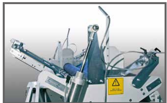
cradle with extensions for loading and unloading (Image 4)
