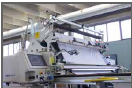
Spreading machine 600 D / E with steam lance
