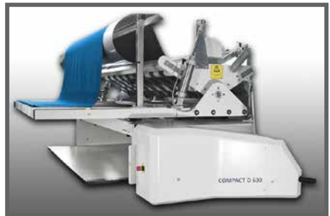
Halfmoon device and platform for folded fabrics (Image 3)
